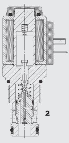
When the solenoid coil is de-energized, the valve blocks flow in both directions. When energized the valve allows flow in both directions. 2/2 Solenoid Directional Valve Poppet Type, Pilot Operated Normally Closed Metric Cartridge Valve – 350 bar WSM12120W
