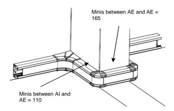
Mini dimension in mm to be respected allowing the installation of angle inter/exter: (in the case of a skirting of post for example)
