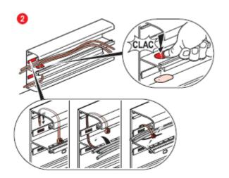
The "t-piece" in the content of the trunking are provided with holes allowing the passage of a collar for the reserve of the cables inside the compartment:
