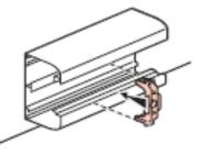
By removing the part of completion of the cover joint, that gives access simply the cover to withdraw it and facilitates the intervention in the compartment.
