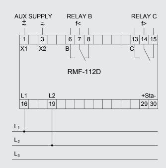
Shown contact positions: Aux. voltage not connected
