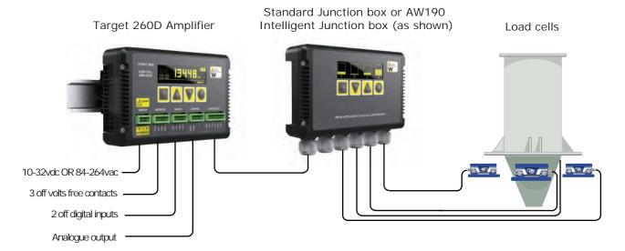
The Target 260 will display error messages for cable break and when used in conjunction with the AW190 Intelligent Load Cell junction box each load cell can be individually monitored for errors or fault conditions. These are displayed on the Target 260 screen. These faults include Cable breaks, Over/Under range and Out of Balance loading on the cells.
