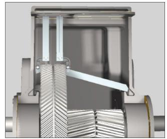
Consistent lubrication is essential even at low speed operation (below 5 SPM). This can be accomplished with the addition of optional high speed gear wipers for reducer sizes 912 and below. High speed gear wipers are standard equipment on reducer sizes 1280 and above.
