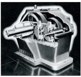
As long as the oil is maintained at the proper level, the slow speed and high speed gears dip in oil and provide continuous lubrication to the gear mesh. Large oil wipers direct a flood of oil into oversized oil troughs which in turn provide each individual bearing with more than adequate lubrication above five SPM
