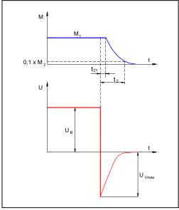
$\mathsf{U}_\mathsf{B}$ operating voltage (coil voltage) Uvmax disconnection voltage
