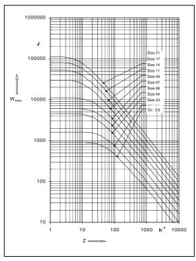
Fig. 24/1: Max. switching work W<sub>max</sub> per switching operation as a function of the number of switching operations per hour Z (values based on n=1000 rpm)
