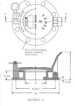
**Example:** Model Number 43108A is a 4310 Series sampling and gauging hatch with 8" aluminum base and cover, NBR insert, flat face flange drilled to ANSI 150.
