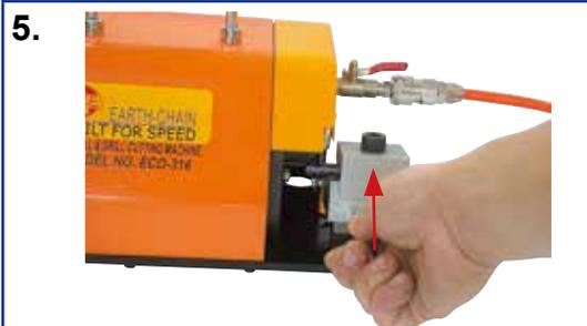
7. Hold and raise the handle to cut off the end mill (drill).
