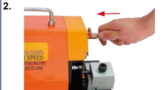
3. Lock the valve connector, then insert the pressurized blast connector into the air pressurized cooling system.
