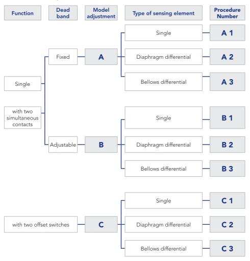
**Note:** Instruments equipped with two simultaneous contacts are adjusted in the same way as devices with a single electrical function.
