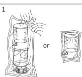
Open the Stericup® or Steritop® bag at the notched edge. The Stericup® filter funnel is packaged fully tightened onto the bottle and requires no further tightening.
